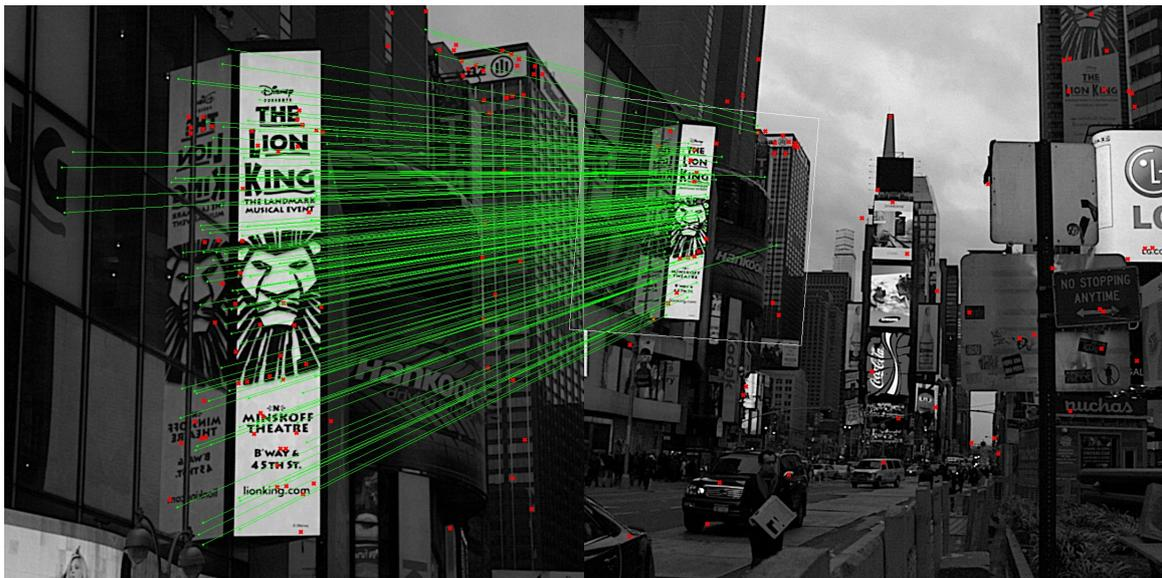
FIG. 9: The left image is aligned with it's location in the right image. The red dots show descriptors extracted with SURF and the green lines show the matched inliers.
